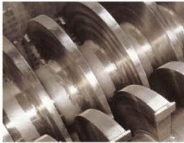
K-S offers a variety of finishes to meet food, pharmaceutical and fine chemical application standards that require polished surfaces and welds.
